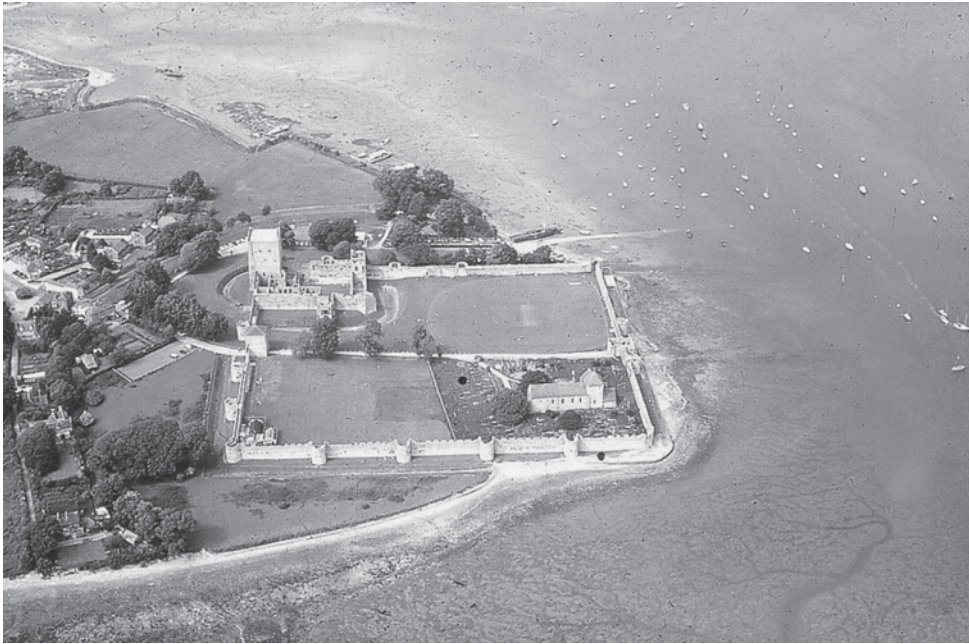
Figure 1 Portchester Saxon Shore fort from the air. The wall surrounding the fort is 10 ft thick and over 20 ft high. The rectangular structure in the top left-hand corner is a medieval castle which was built to make use of a small part of the surviving Roman walls.
