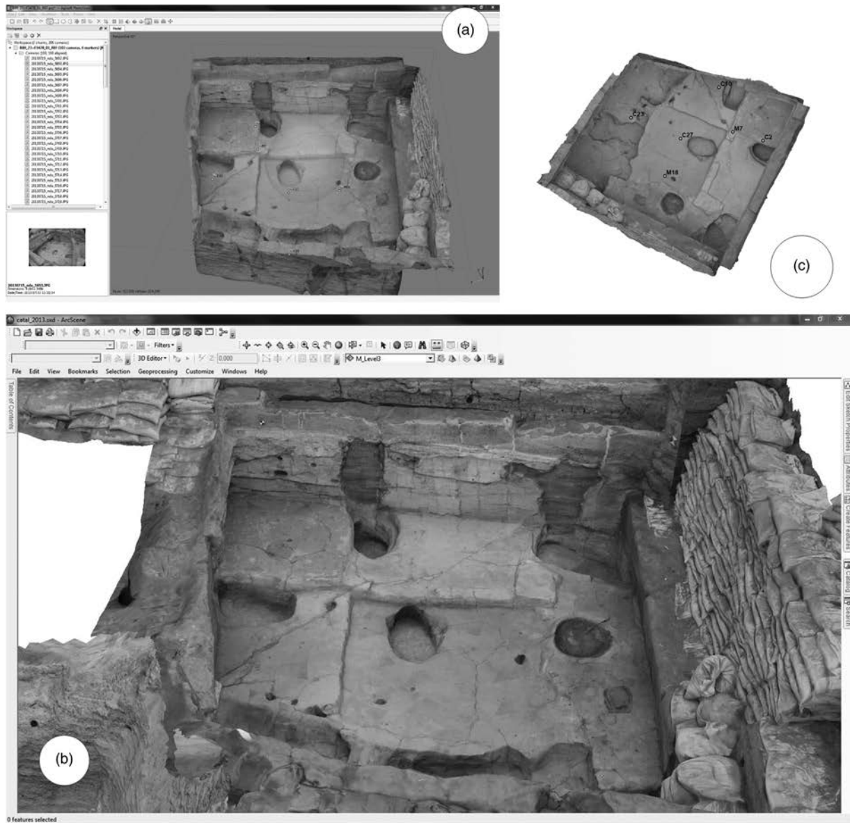
Figure 3. 3D surface model of B.89 generated in Agisoft Photoscan (a) and implemented in the 3D GIS (b) using GCPs (c) to georeference the model.
