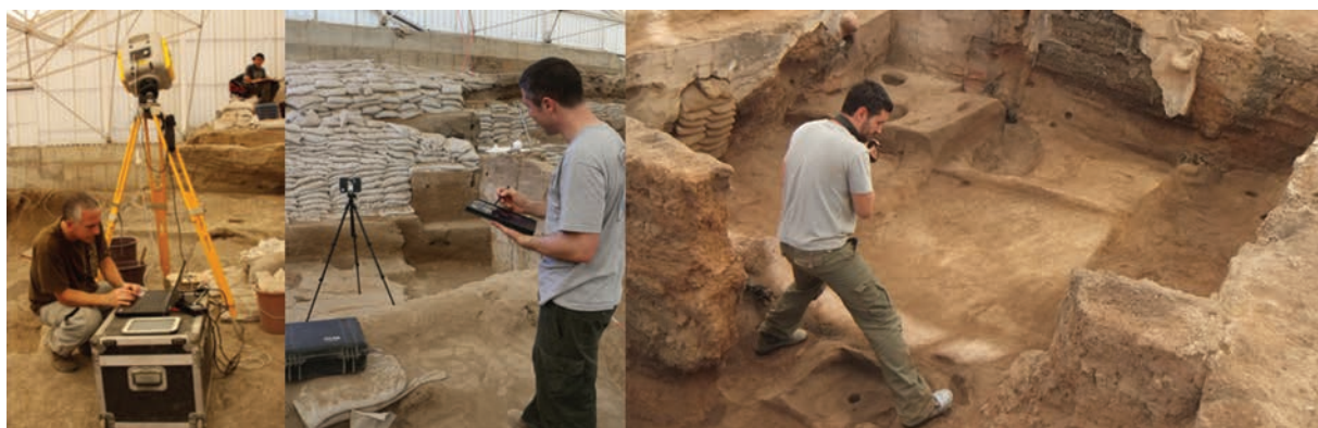
Figure 1. Data capturing sessions via laser scanning and image-based 3D modelling. Courtesy of the 3D-Digging at Çatalhöyük project team.
