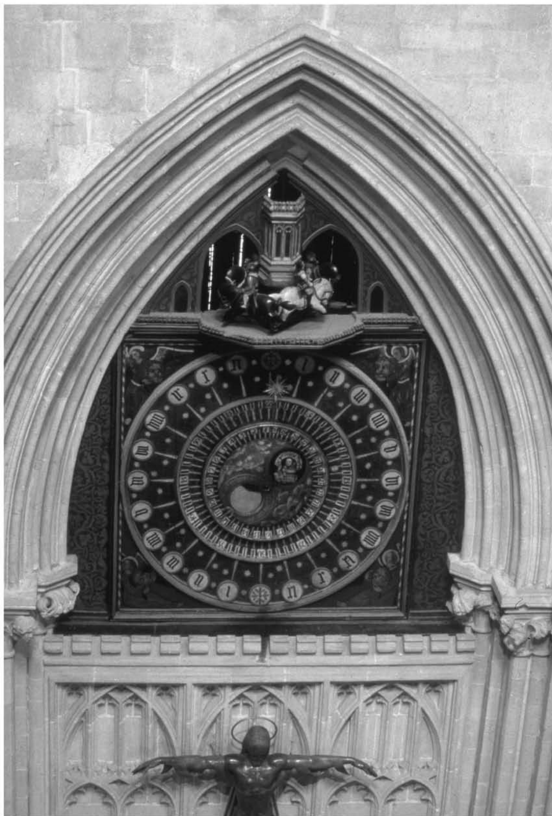
Plate 24 Technology: The Cathedral Clock, late fourteenth century, showing the dial which portrays hours, minutes, position of the sun, date of the lunar month and the phases of the moon
