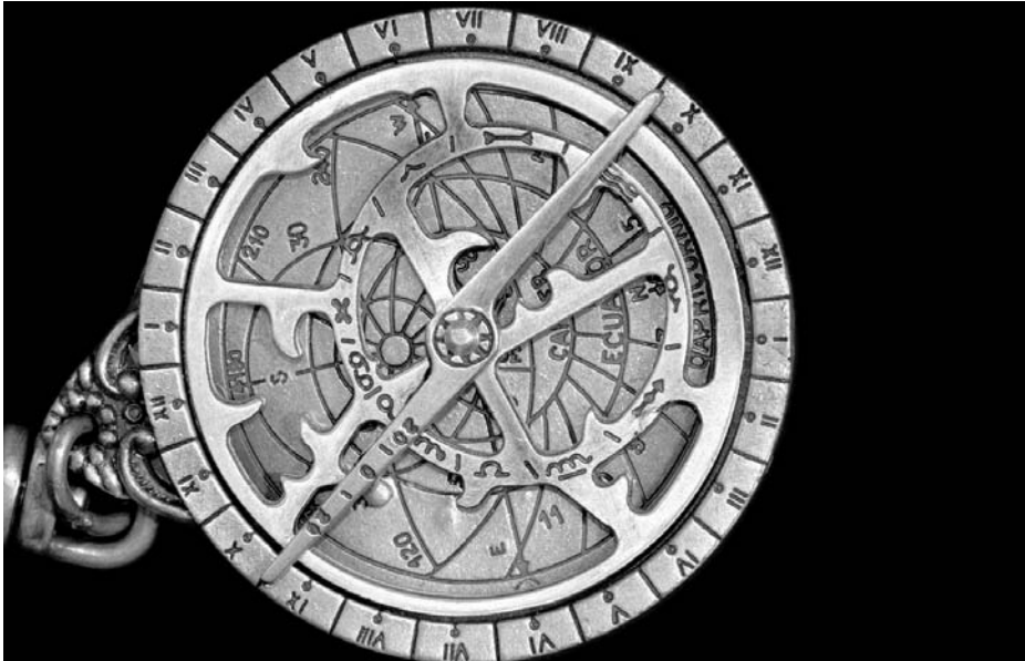
The astrolabe was the first instrument to represent both time and space as a circle divided into 24 units. (Brian Maudsley)
