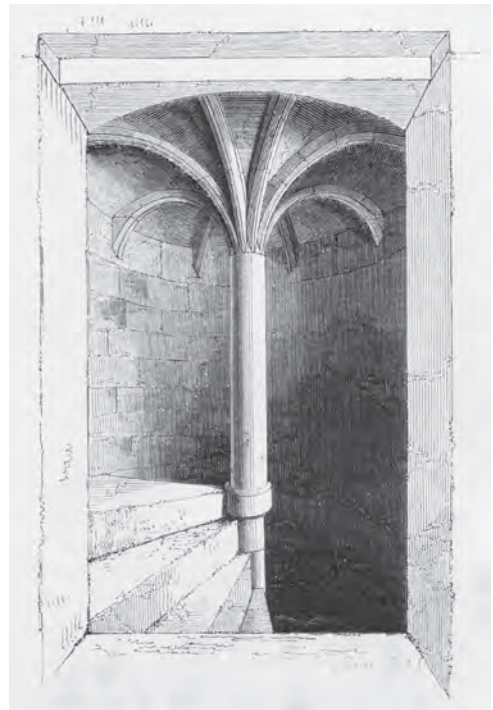
Fig. 4.26. Alnwick (Northumberland) Umbrella vault over a staircase (c. 1370); from Hartshorne 1858
