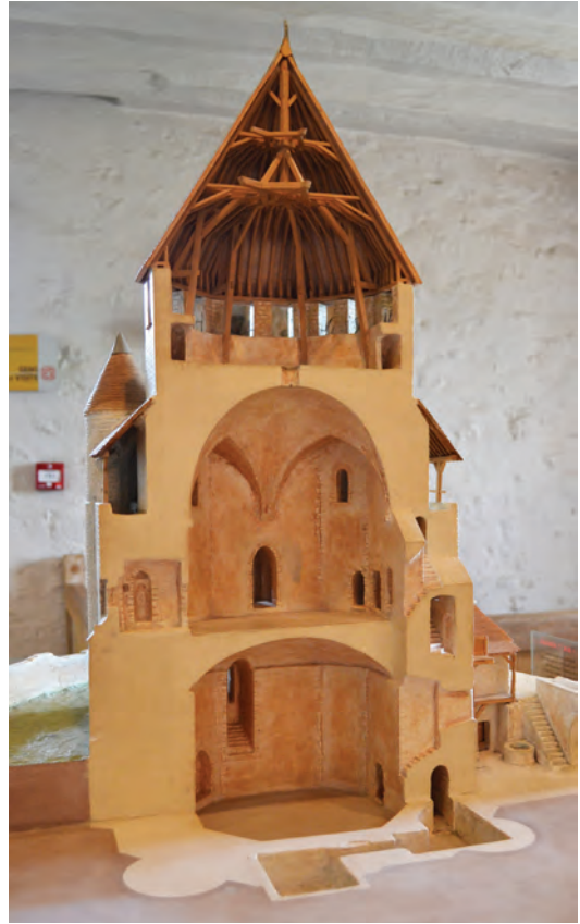
Fig. 3.9. Provins (Seine-et-Marne) Sectioned model of the Tour de César showing the eastern half of the building (third quarter of the twelfth century).
