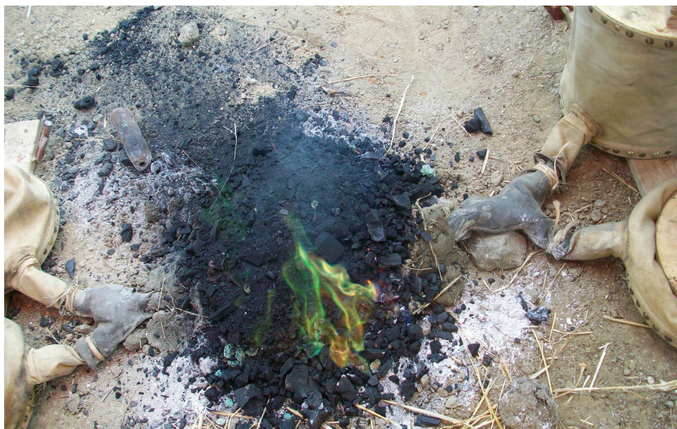
Figure 2.6 Green flames during copper smelting.
