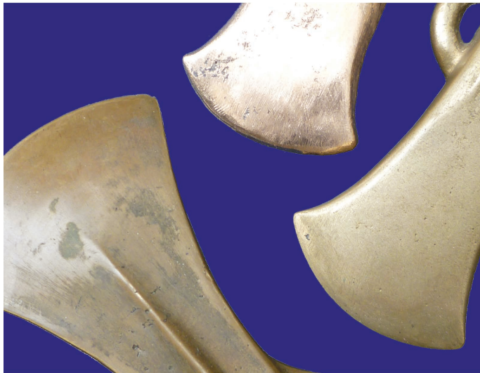
Figure 3.5 Three bronze axeheads of differing ages. Top: This axehead, approximately a year old, retains its shine and colour. Right: This example, at five years old, has a visibly duller surface with a slightly darker colouration. Left: This axehead, at ten years old, has a duller and darker blade, with regions of deposited corrosion product.
