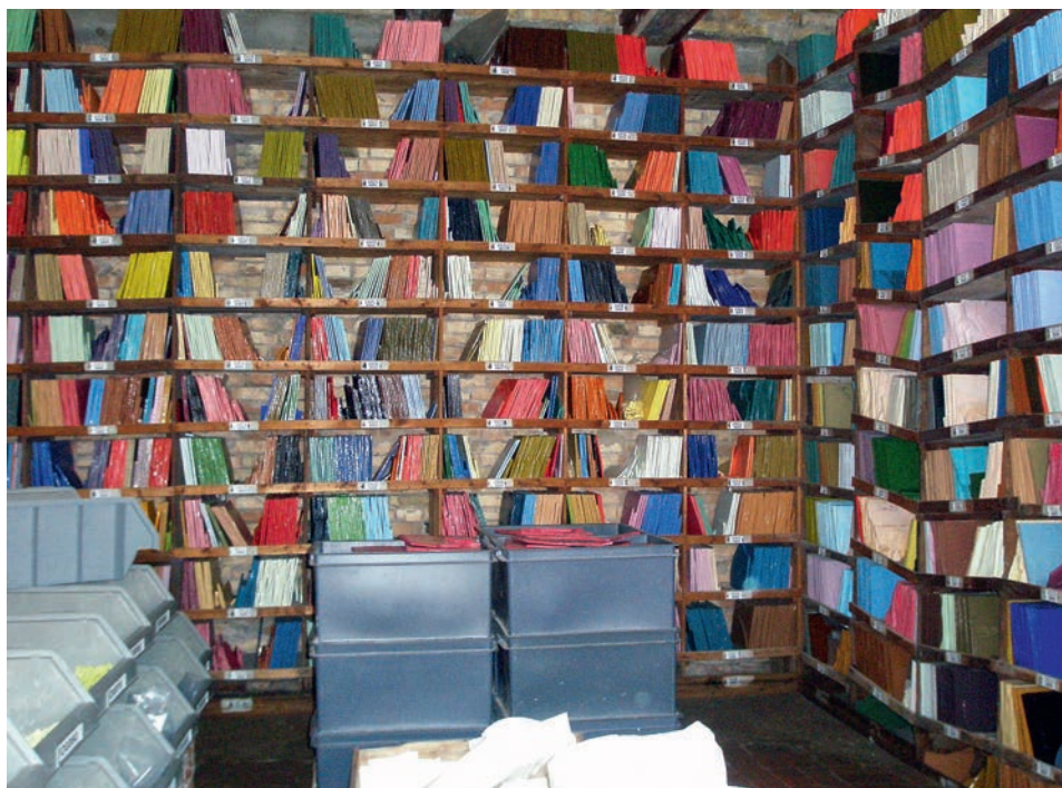
Figure 9 Sheets of coloured glass for making tesserae in the Orsoni Factory, Venice: this range of colours owes much to modern industrial techniques.
