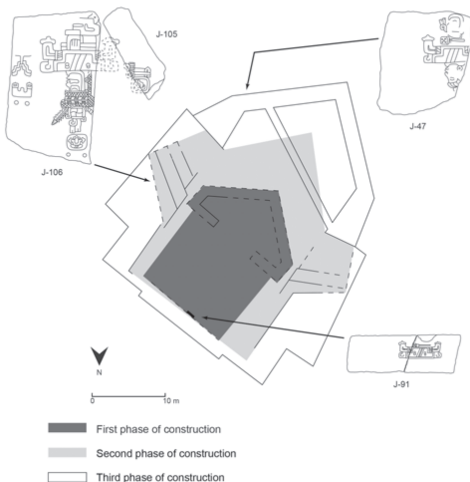
FIGURE 9.6. The three main construction phases of Building J. The finely incised orthostats, many of them already fragmented and eroded, were reused beginning with the first version of the building. Drawing by Elbis Domínguez Covarrubias.
