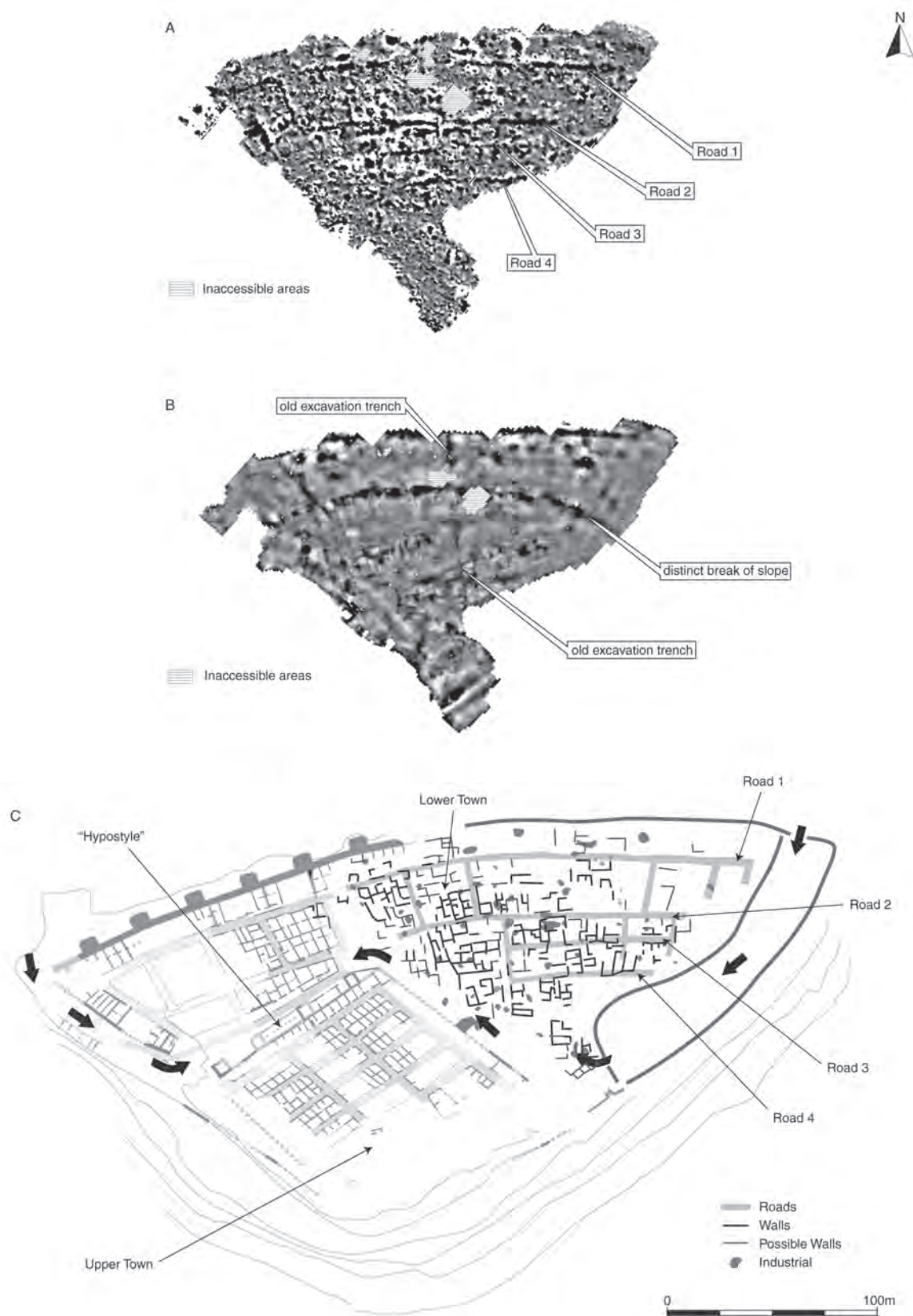
Fig. 15.8: Entremont: (a) magnetic data; (b) earth resistance data; (c) interpretation of the combined data-sets (authors)
