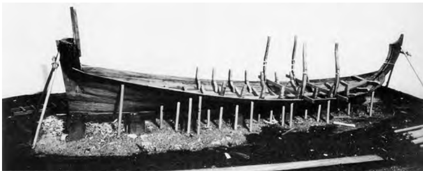
FIGURE 3.8. Futtocks are raised at several locations. To check the overhang of the frames, measurements are taken from the line stretched between stem and stern and lines stretched between the port and starboard parts of the frames, combined with measurements taken with a plumb line. In model building this practice is almost impossible unless the model is mounted securely on a board. (Courtesy A. J. Hoving)
