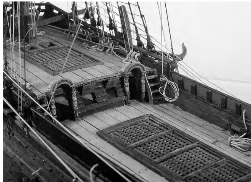
FIGURE 2.200. The forecastle deck of the pinas model. In the forecastle bulwark the ports are visible, through which the messenger runs to the capstan. The boat that is normally stowed on the gratings has been removed for the photograph (cf. fig. 2.219). (Courtesy Cees de Jonge, The Visual Art Box)
