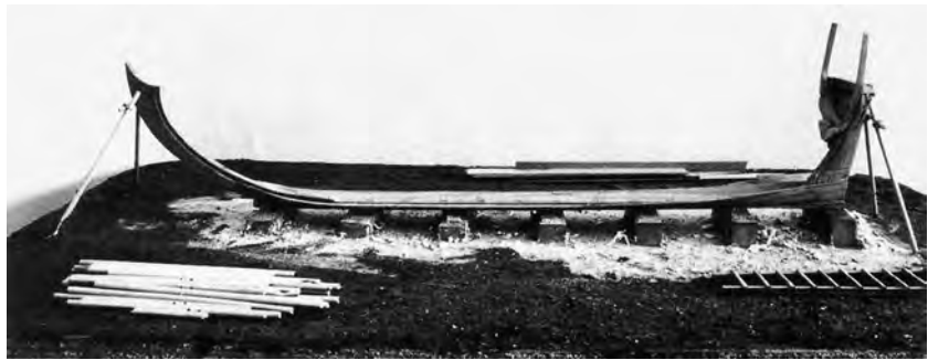
FIGURE 3.3. The first stage of the building process: keel, stem, and sternpost are joined to form the backbone of the ship. The first planks, the garboard strakes, have been fitted. (Courtesy A. J. Hoving)
