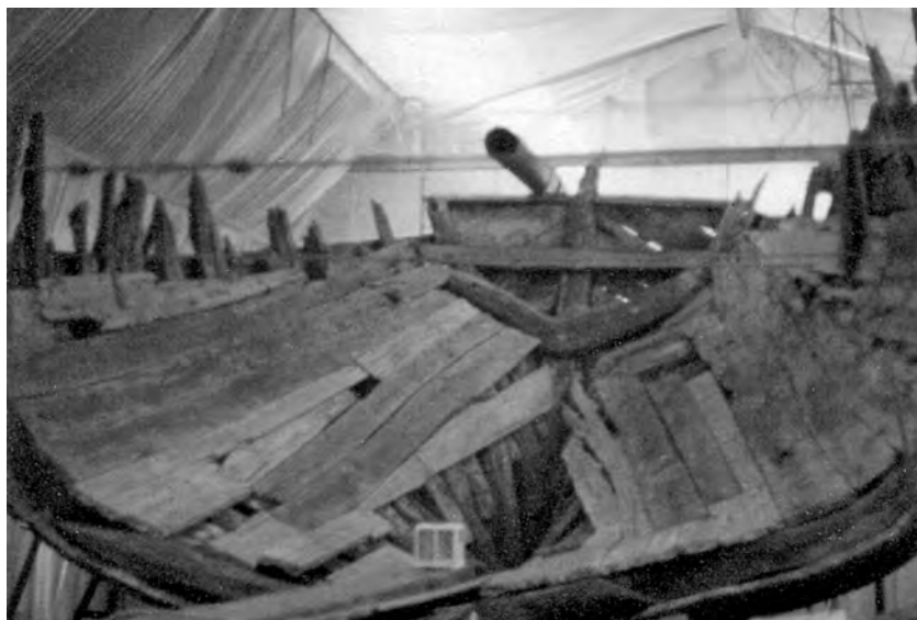
FIGURE 2.69. Ceiling planks in the wreck of a seventeenth-century trader. Apparently the builder was not very careful in the choice and the neatness of his material. (Photograph by A. J. Hoving)
