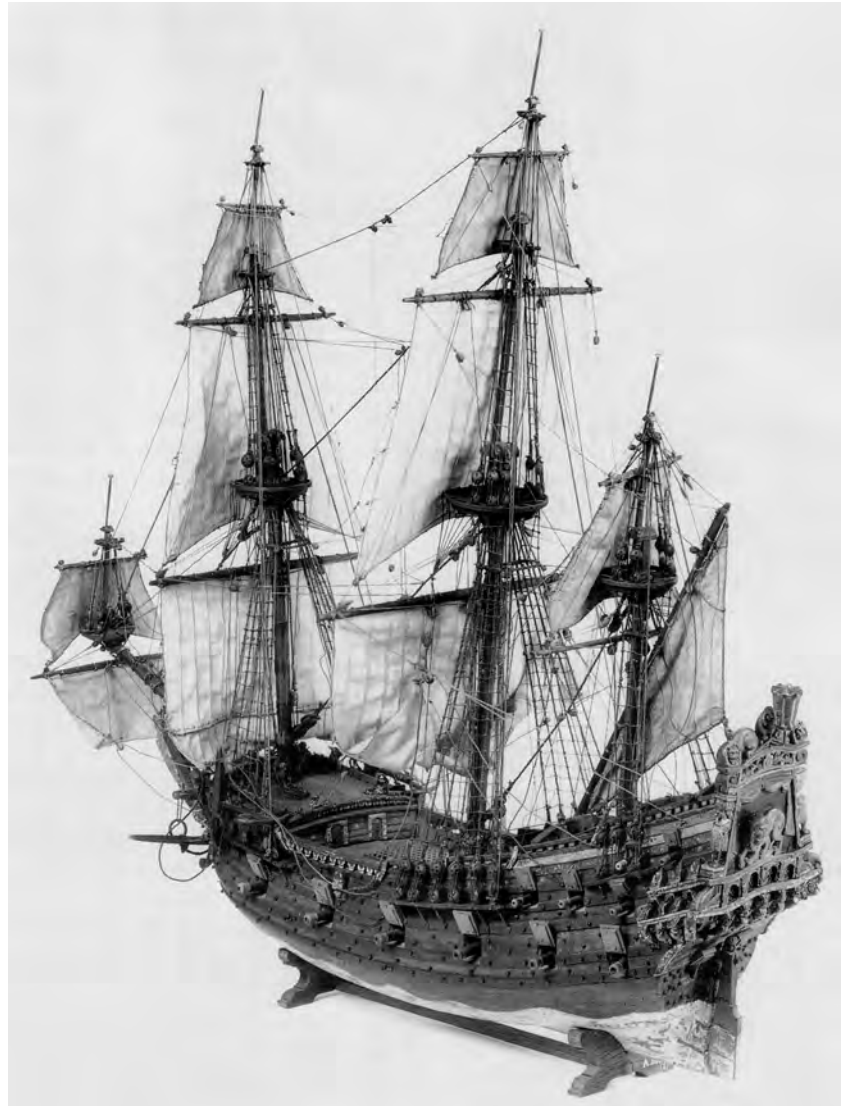
FIGURE 1.8. Model of a pinas, or war yacht, from the mid-1700s. The model was hung in a church for decoration, which is why the underwater part of the hull is not to scale. Yet it gives a fair image of the pinas of that period. (Courtesy Het Scheepvaartmuseum, Amsterdam)
