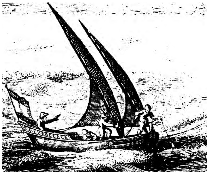
FIGURE 3.13. Detail of a print by Claes Janszoon Visscher, c. 1635. On boats with the mastless “lateen yard rig” depicted here, the sails were probably never lowered but furled around the yard with the sheet. They were probably marled to the yards with a lacing line, and the yards would have to be lifted from the tabernacle to remove the sail altogether.
