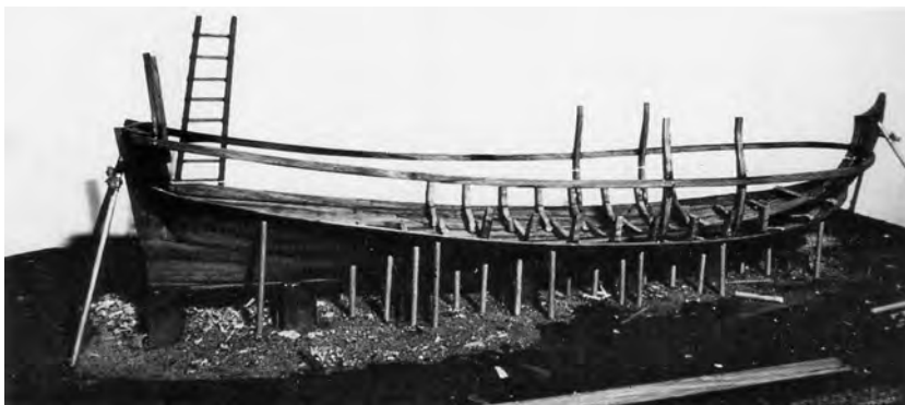
FIGURE 3.9. The master ribband is positioned from stem to wing transom along the futtocks. This temporary ribband was very important, as it indicated not only the maximum breadth of the hull but also the height of breadth and the sheer. (Courtesy A. J. Hoving)
