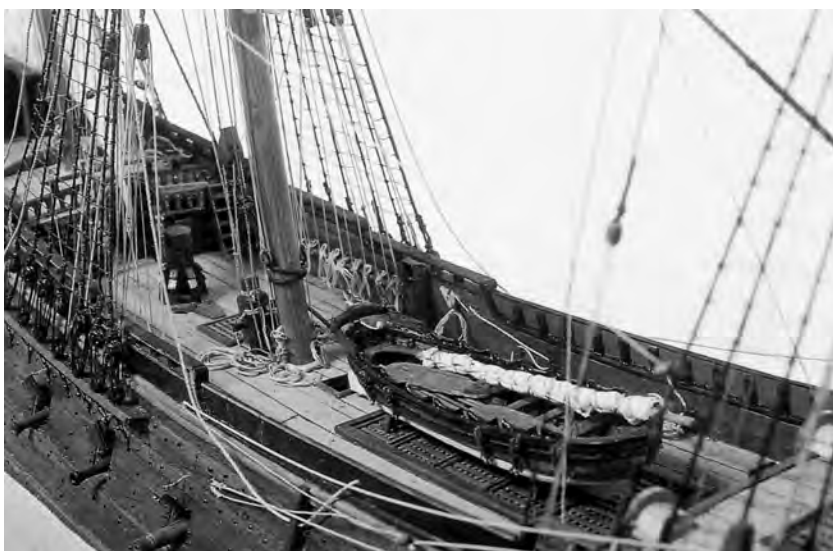
FIGURE 2.219. The waist of the pinas model. The capstan, the knight heads, the boat on the gratings, and the chesstree are clearly visible. (Courtesy Cees de Jonge, The Visual Art Box)
