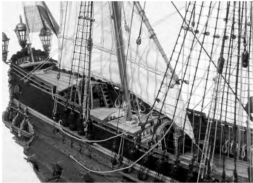
FIGURE 2.199. The quarterdeck of the pinas model. The bulwarks for the steering stand and cabin are visible, as is the arch for the whipstaff (see section 119, Arch above the Whipsta , if necessary). At the aft end of the poop deck we see the bench, which also serves as a chicken coop. (Courtesy Cees de Jonge, The Visual Art Box)
