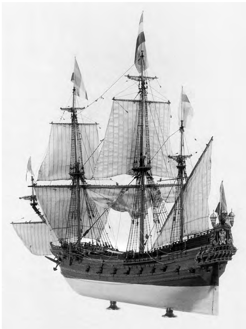
Figure 1.9. Model of a pinas, built by the author from information in Witsen's treatise. Originally a small war jacht, the pinas developed into an armed merchantman of medium size in the middle of the seventeenth century, later into a heavy East Indiaman. (Courtesy Cees de Jonge, The Visual Art Box)
