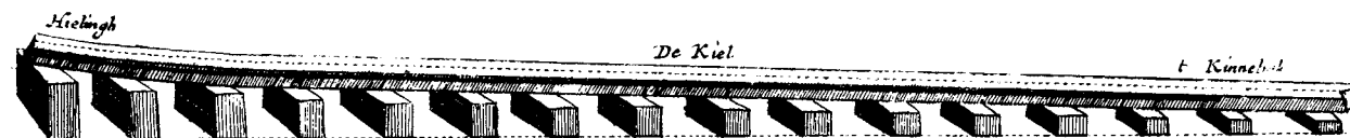
FIGURE 2.2. Plate XXVIII. The keel. Left , heel (i.e., aft end of keel); right , boxing scarf (lit., "jawbone")
