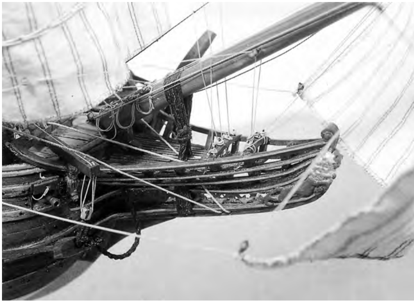
FIGURE 2.165. The beakhead on the pinas model. (Courtesy Cees de Jonge, The Visual Art Box)
