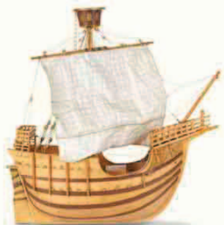
SPANISH COCCA (1450) The Mediterranean equivalent of the cog was the cocca. It had a broad, rounded hull to maximize space for cargo and a crow's nest on its main mast.
