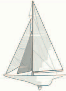
J-CLASS RULE (1930–37) These beautiful bermuda-rigged yachts had unlimited sail area, but a fixed draft (depth of keel) and length.
