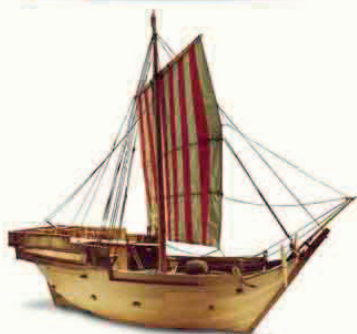
BREMEN COG (1380) The cog was the standard northern European ship during the Middle Ages. It had a single mast, a square sail, and a spar projecting from the bow to anchor the sail.
