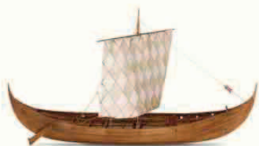
VIKING KNORR (c.1000) The knorr was the type of cargo ship that the Vikings used to colonize Iceland, Greenland, and eventually Vinland. It was typically 56 ft (17 m) long and 15 ft (4.5 m) wide.
