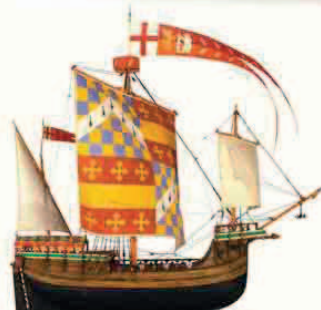
ENGLISH COG (1485) By the mid 15th century, the ships had "castles" fore and aft, which served as excellent platforms for bowmen in times of war.
