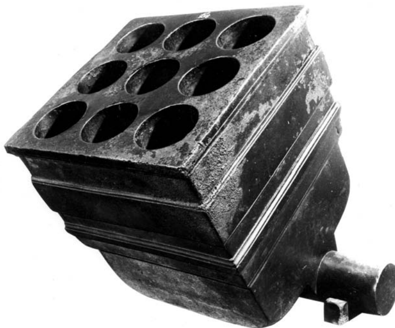
Figure 14.6. Nine chambered bronze mortar, designed by Richard Leake and cast by William and Philip Whiteman, London 1687 (Tower of London, inv. XIX.131, © Board of Trustees of the Royal Armouries).
