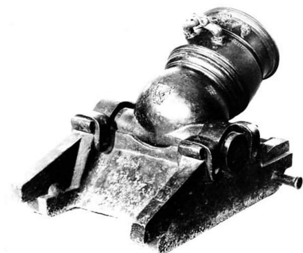
Figure 14.1. Bronze 12-inch mortar and iron bed, Spanish, dated 1724. Cast by Voie-Y-Abet of Seville, gourd shaped chamber (Tower of London, XIX.142, © Board of trustees of the Royal Armouries).
