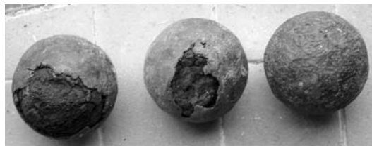
d) Lead coated wrought iron shots for the passavolanti, re-employed in a bronze demi culverin found in the Sciacca wreck (Photo: Soprintendenza di Agrigento).
