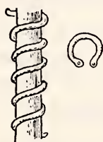
FIG. 1. Probable method of making links for mail.
